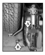
3. Tighten the wingnut (A) until the jack is securely fastened.
